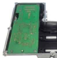
Fig.32. Partial detail of PCB assembly of aluminum for an On Board Charger (OBC) in electric vehicles.
