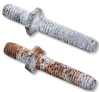
Fig.49. White corrosion and red corrosion appearance.
