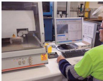
Fig.48. Measurement of layer thickness by X-rays.
