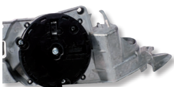
Fig.31. Rear-view mirror motor assembled on aluminum housing.
