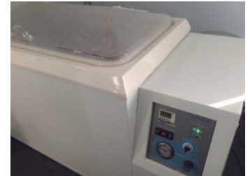
Fig.50. The test in Salt Spray Chamber are made based on Control Plan.
