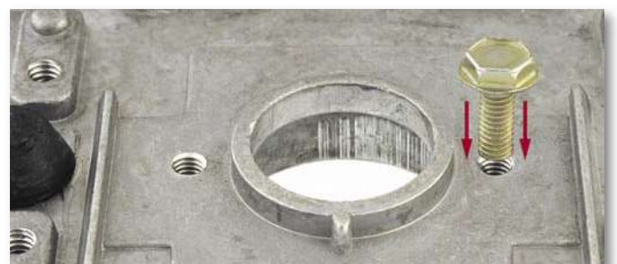
Figure 20 In parts with a large number of holes, pre-operational costs become sky-high.
