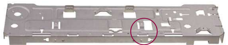
Figure 55 During metal sheet mechanisation with many holes and folds, small dimensional variations cause hole misalignment.
