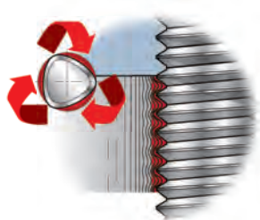
Fig.29. The material displacement during threading flows between the lobes wrapping the shank of the screw.
