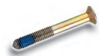
Fig.44. The adhesive patch loses a large part of its locking properties and wears away when exposed to high temperatures. The screw cannot be reused and assembly costs are high.
